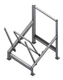
A rack designed to ensure that the liferaft will immediately drop into the water without assistance. For throw overboard liferafts weighting more than 185 kg sliding ramps are mandatory, in accordance with the SOLAS convention chapter III regulation 16. Pre-drilled foundation holes have a diameter of Ø14.
